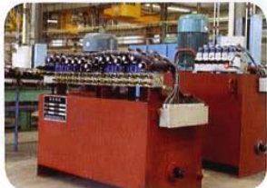
液压泵站 Hydraulic pump station
