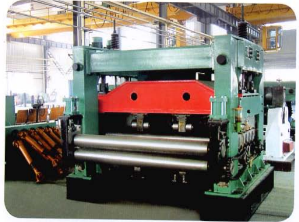
WB43M-10×2000( \delta \leq 450\text{MPa} ) 矫平机用于青岛造船厂 Plate straightening machine used for Qingdao Ship Building Factory.
