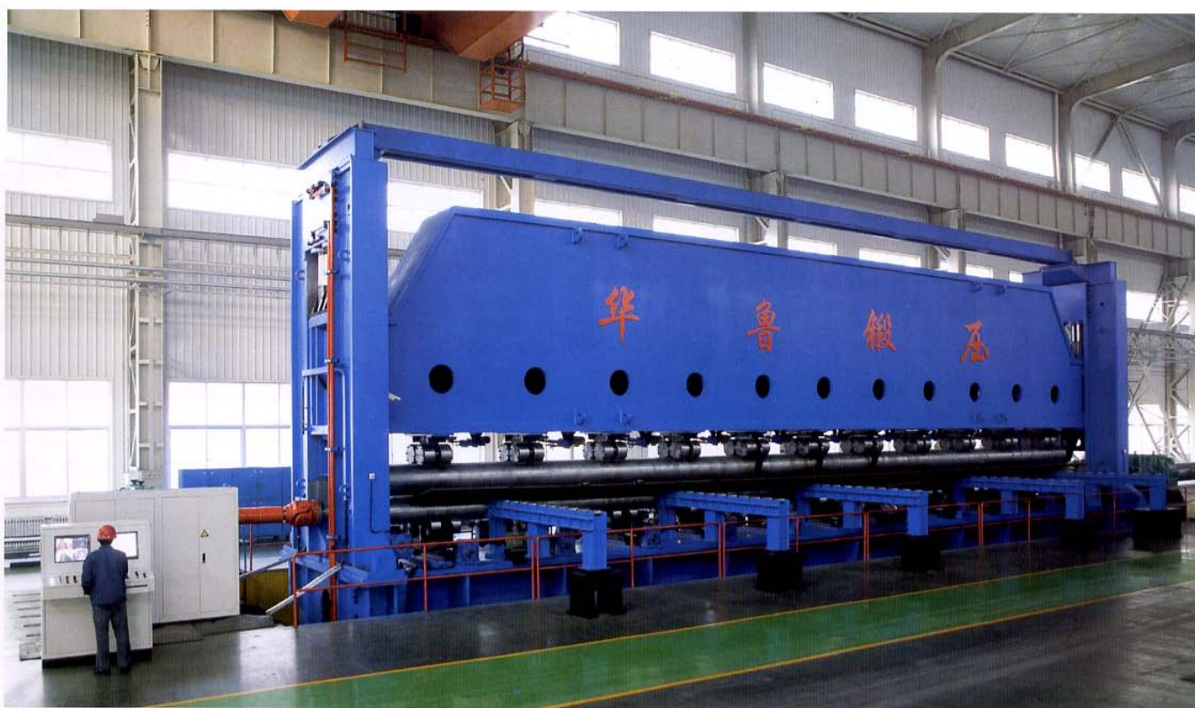
WEF11K-35 × 21000 CNC shipyard plate bending machine for Jinhaiwan Shipyard Co., Ltd., zhongji Shipyard Co., Ltd.
