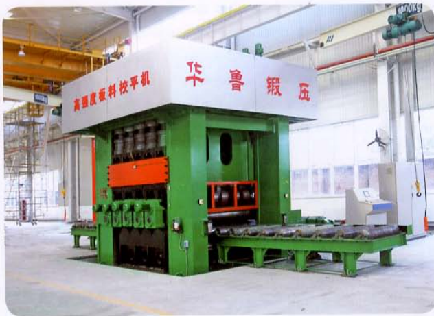
WD43M-40×2000 ( \delta \leq 690\text{MPa} ) 矫平机用于中煤北京煤矿机械有限公司 Plate straightening machine for China Coal Beijing Coal Mining Machinery Co., Ltd.
