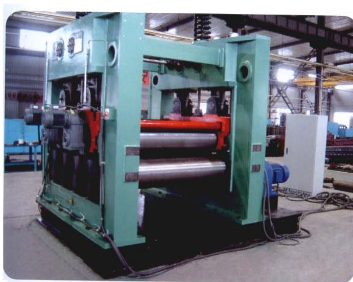
WC43-32 × 1300 ( \delta \leq 360\text{MPa} ) 矫平机出口俄罗斯 Plate straightening machine exported to Russia
