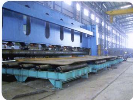
WE11N-35×13500 船用卷板机用于越南下龙船厂 Marine rolling machine is used in Vietnam Halong Ship Building Enterprise
