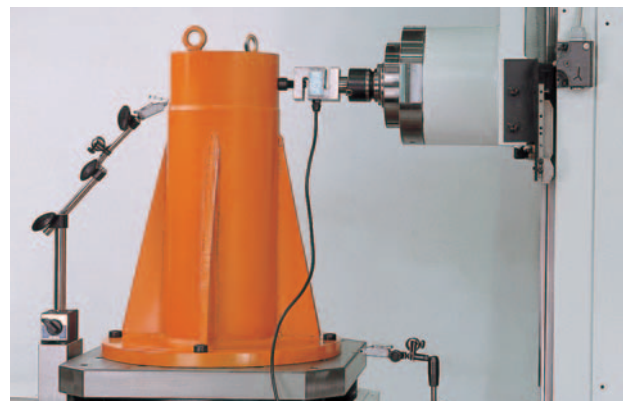
Load cell test to guarantee the rigidity
