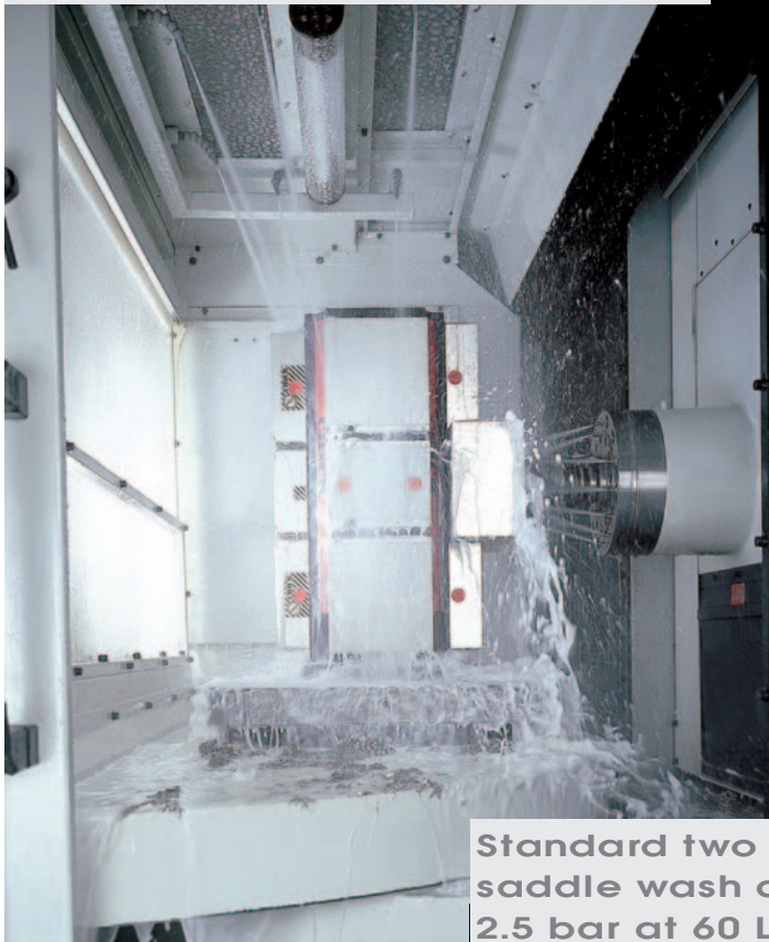
Standard pallet wash system (Ceiling wash down) 0.8 bar at 60 L/min.
