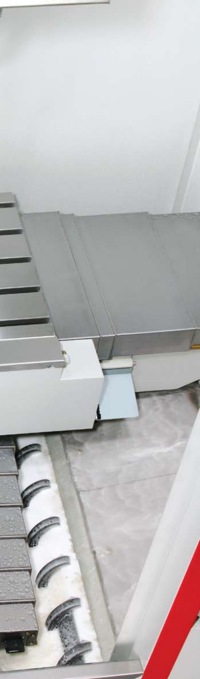
Better chip flow by augers direct to the rear
