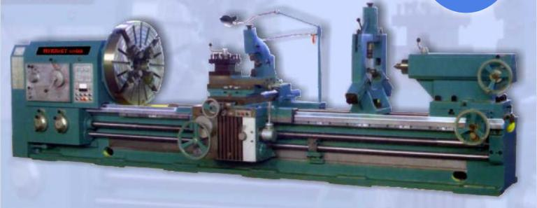
CW61100B, CW61125B, CW61160B parallel lathes are suitable for turning of cast iron and steel workpieces, turning of non-ferrous metal parts of big or medium sizes. It can do external cylindrical surface turning, inner hole and end face turning. It can also turn various internal and external metric, inch module and diamerical pitch threads, the top slide can be used independently for turning of short taper.
