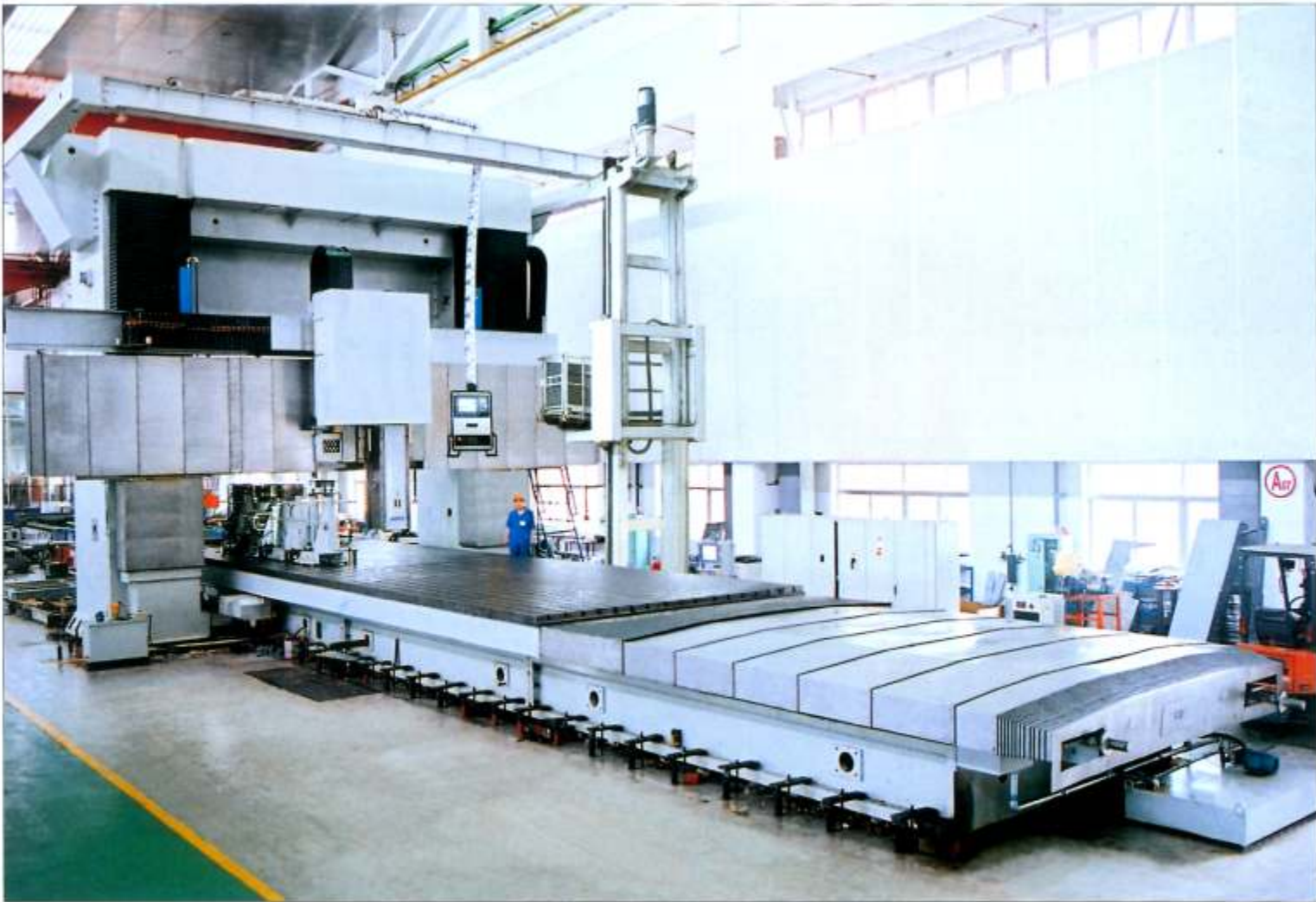
• XK2145 gantry type CNC boring & milling machine with movable crossrail, table travelling
