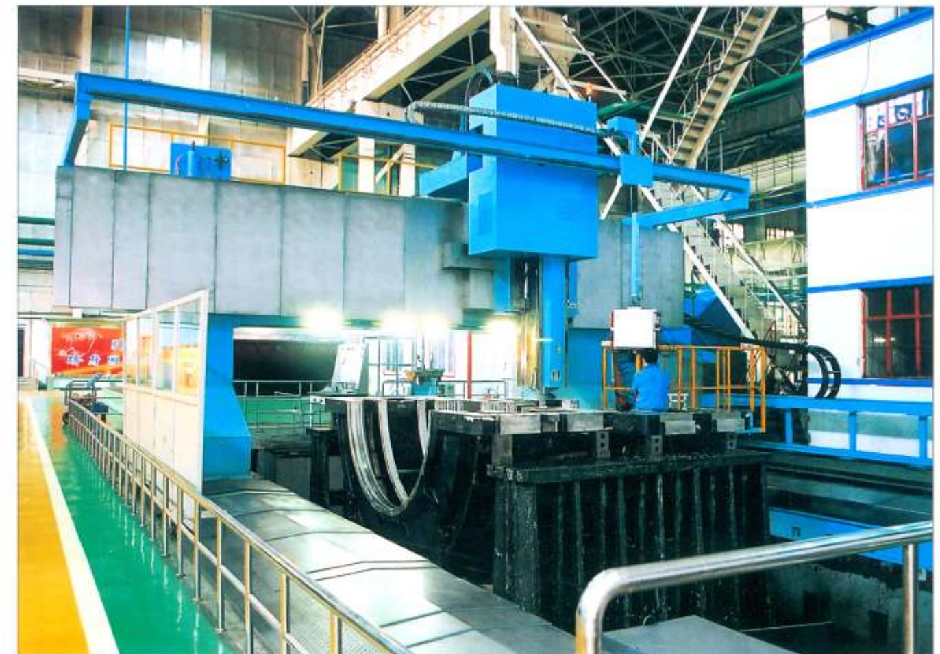
• XK2745 gantry type CNC boring & milling machine with fixed crossrail, gantry travelling
