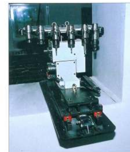
• A disk type tool magazine of cap. 20 pcs
