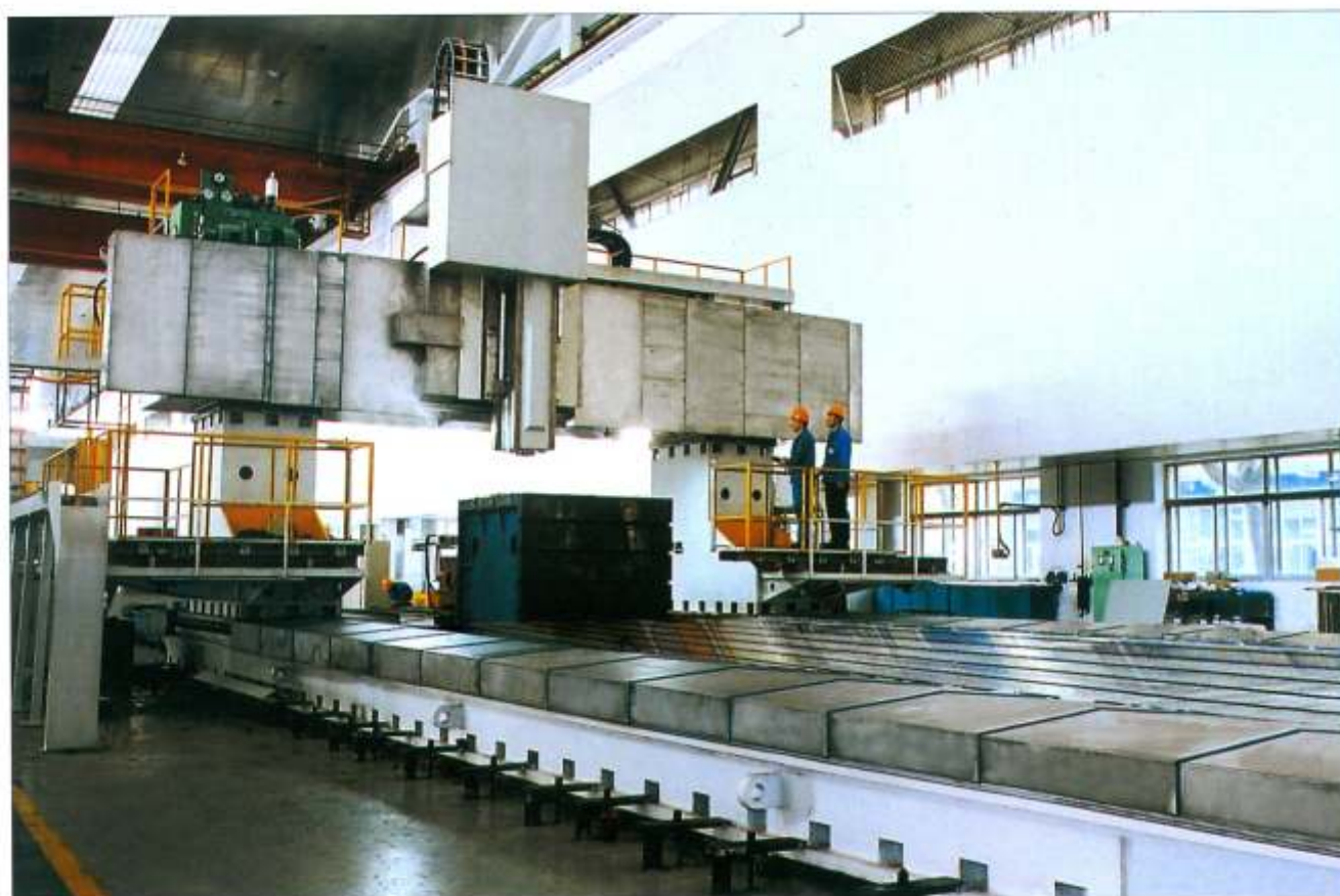
• XK2740 gantry type CNC boring & milling machine with fixed crossrail, gantry travelling
