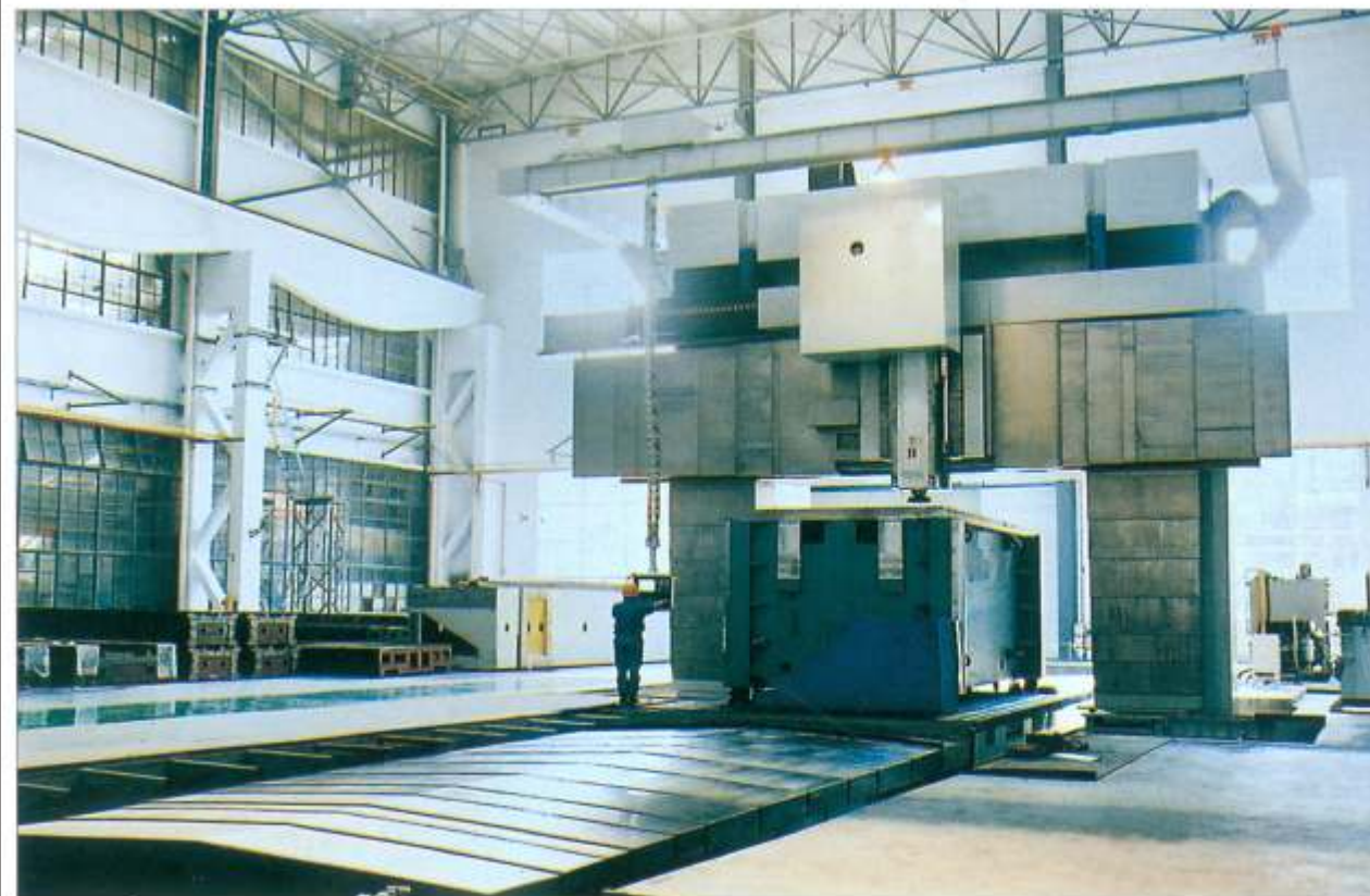
• XK2140 gantry type CNC boring & milling machine with movable crossrail, table travelling
