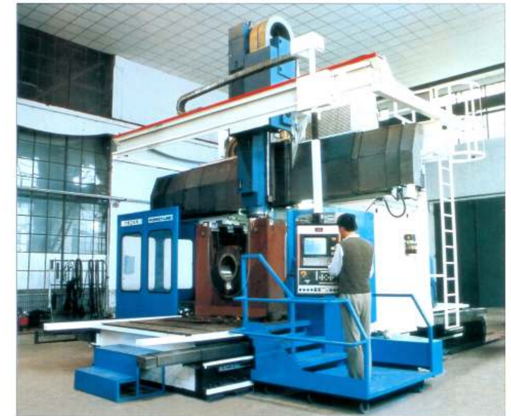
• XH2720 gantry type machining center with fixed crossrail, gantry travelling
