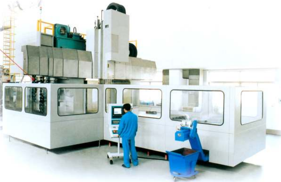
• XH2420A gantry type machining center with fixed crossrail, table travelling
