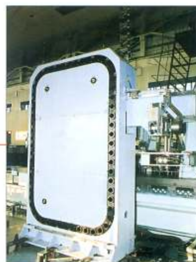
• A chain type tool magazine of cap. 60 pcs
