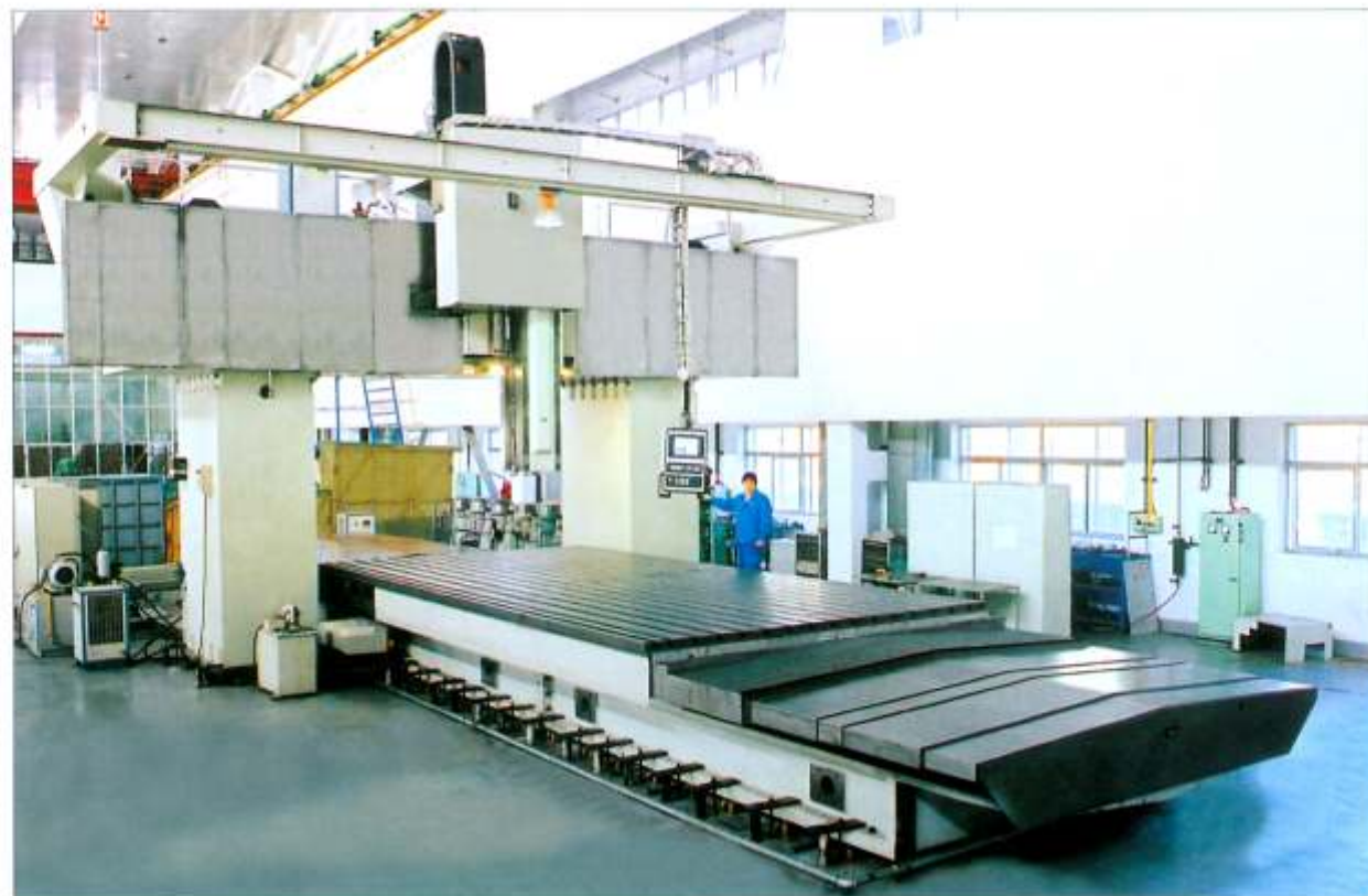
• XK2440 gantry type CNC boring & milling machine with fixed crossrail, table travelling
