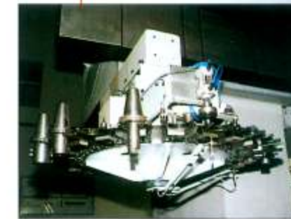
• A disk type tool magazine of cap. 24 pcs
