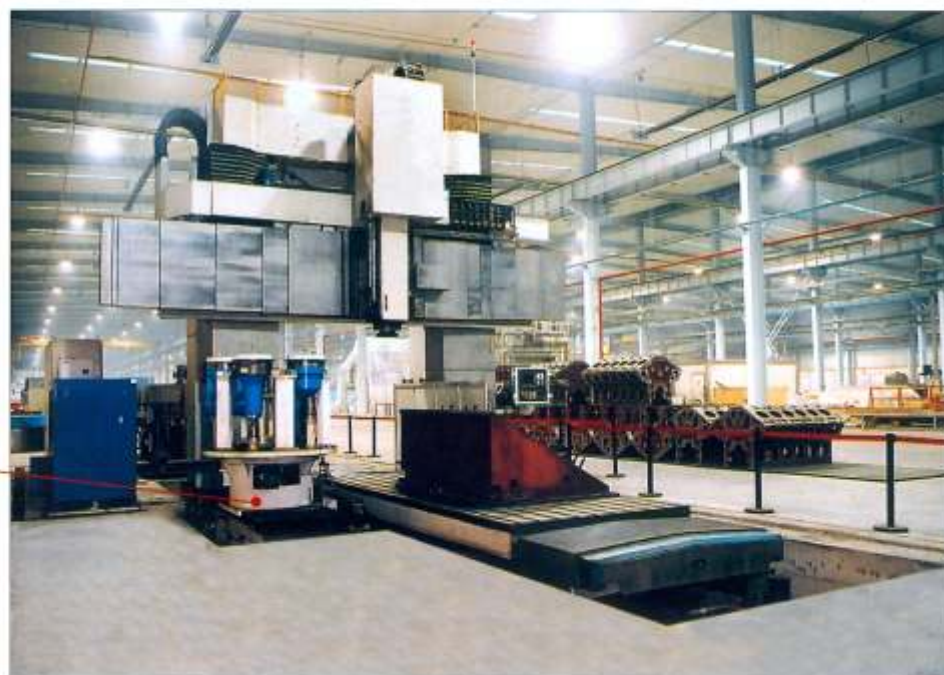
• XH2120 gantry type machining center with movable crossrail, table travelling
