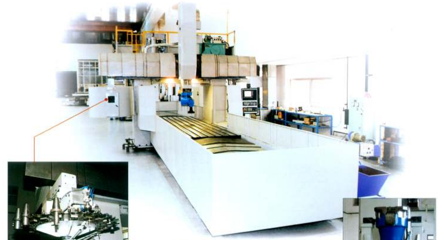
• XH2418 gantry type machining center with fixed crossrail, table travelling
