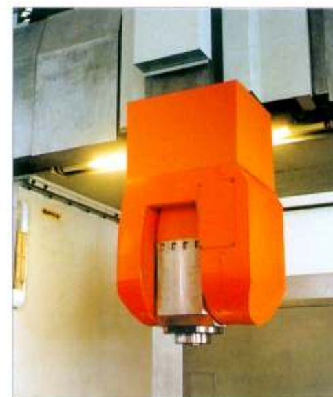
• Mechanical type dual swivelling milling head with large torque
