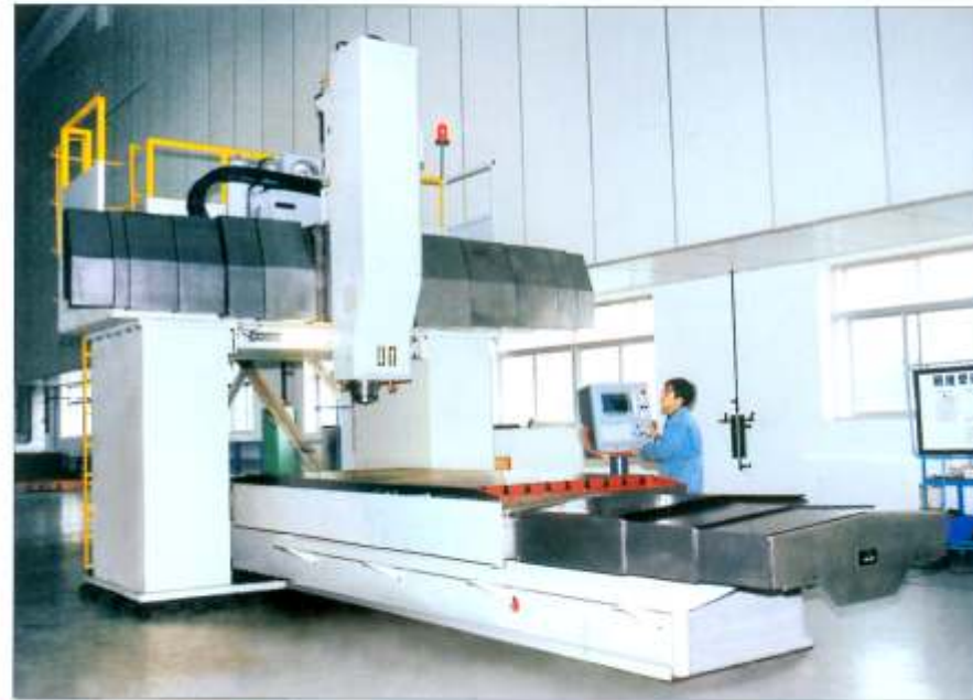
• XK2411 gantry type CNC boring & milling machine with fixed crossrail, table travelling
