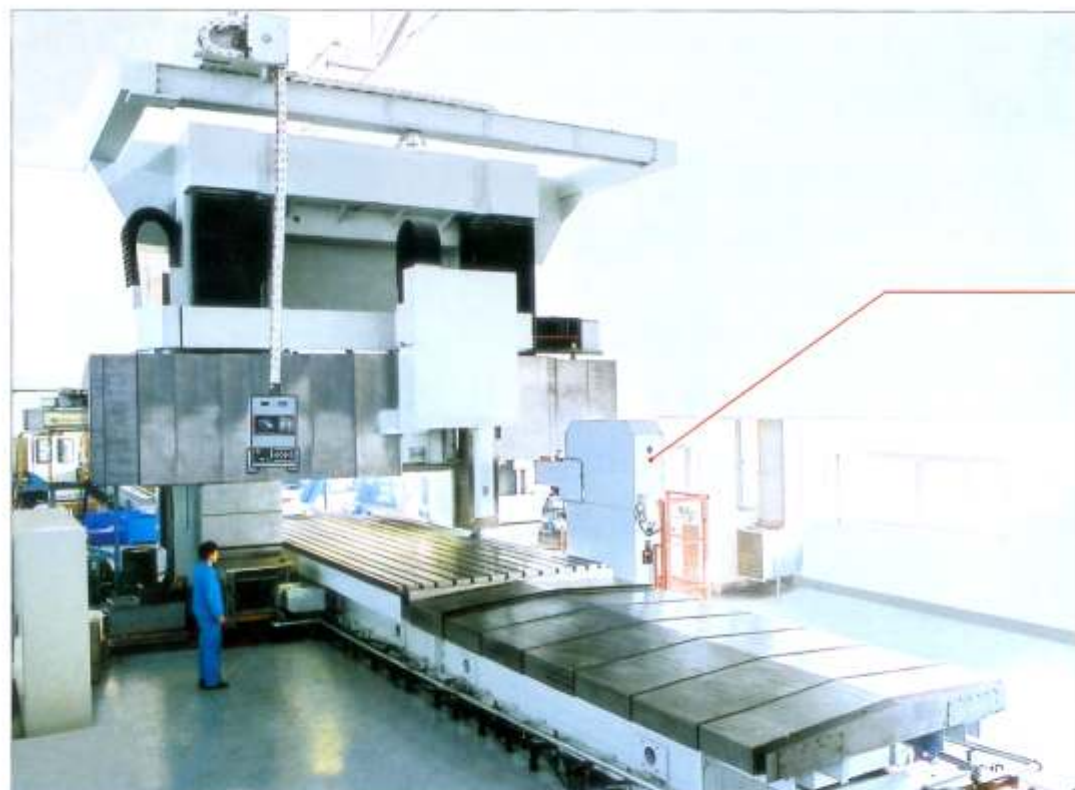
• XH2130 gantry type machining center with movable crossrail, table travelling
