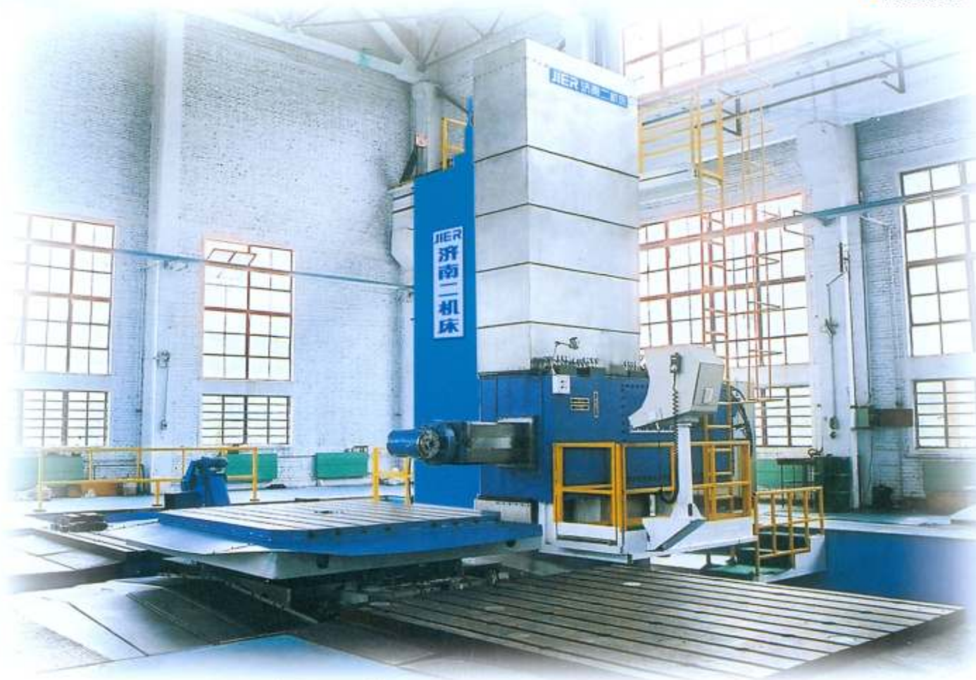
• TK6916 floor type CNC boring & milling machine
