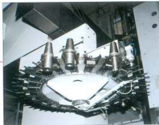
• A disk type tool magazine of cap. 24 pcs
