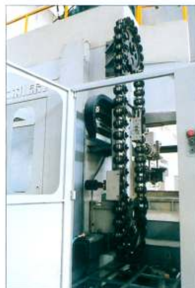
• A chain type tool magazine of cap. 50 pcs
