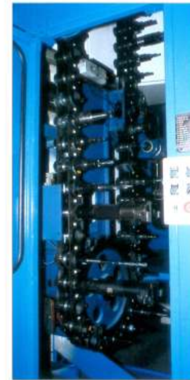
• A chain type tool magazine of cap. 50 pcs
