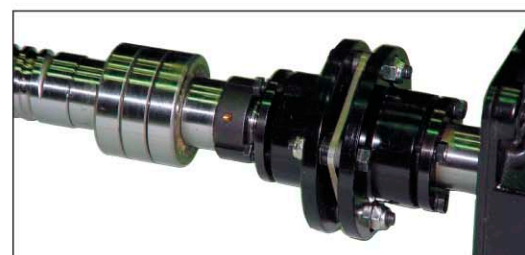
Ballscrew: High precision bearings and coupling are used to support the super precision ballscrews to ensure reliability in positioning.
